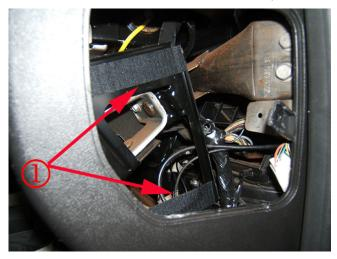
Install the other side of the 2" Velcro® 191195 Reclosable Loop Fastener Tape (hook and loop) or equivalent to the OnStar® module bracket as illustrated. Use the Reclosable Loop Fastener Tape or equivalent to secure the OnStar® module to the bracket.
