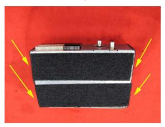
2. Obtain two strips, approximately 177 mm (7 inches) in length, of 2" Velcro® 191195 Reclosable Loop Fastener Tape (hook and loop) or equivalent and apply one side of the tape to the bottom of the module as shown above.
