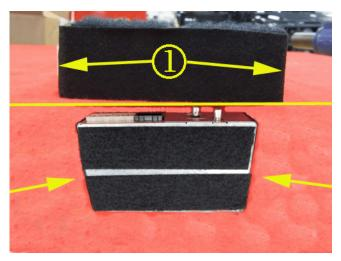
4. Cover both sides of the module with BRS Tape KT13487 (1) or equivalent, as shown above.
