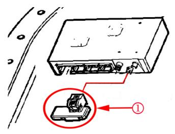
2. If installing the modules P/N 23230482, 23230536, 23230537, 23235220, 23235227, 23235234 and 23383877, transfer the Bluetooth Antenna(1), if equipped, to the new module.
