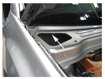
1. Remove the windshield wipers and cowl screen where sealing repair is to be done.
