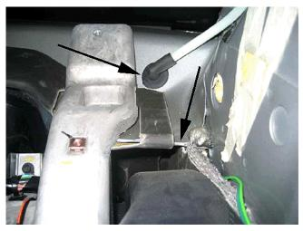
Water from the right front sunroof drain hose exits the vehicle through the plenum (upper arrow) and may re-enter through the un-sealed seam at the front of the dash. Refer to lower arrow in the illustration.
