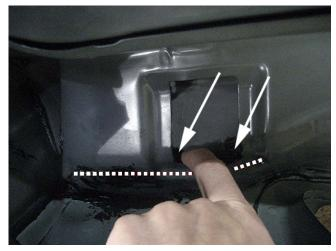
4. Seal the seam INSIDE the opening at the bottom and to the right and left of the arrows in the illustration. Seal the full length of the dotted line. Seal the seam with P/N 12378500 (in Canada, use 10952233) Medium Body Seam Sealing Compound or equivalent.
