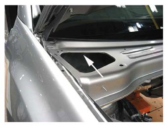
1. Remove the windshield wipers and cowl screen where sealing repair is to be done.
