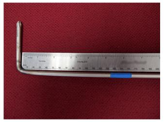
4. Install masking tape on the tool as shown. Place the tape approximately 130 mm (5.2 in) from the 90° bend. The tape on the release tool helps indicate the insertion depth and protects the paint finish on the edge of the hood.
