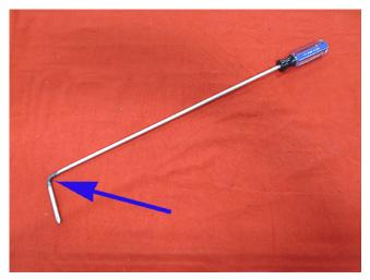
3. Clamp the screwdriver in a vise and create a 90° bend as shown.
