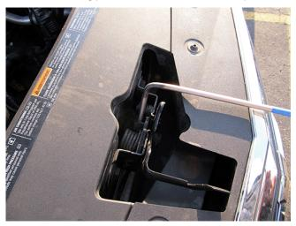
2. Turn end down into the center of the latch.
