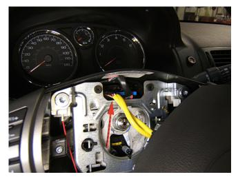
This condition may be caused by a short to ground in the yellow SIR wiring harness. This wiring harness is located within the steering wheel assembly and connects the steering wheel inflatable restraint module to the steering wheel inflatable restraint module coil. A sharp edge on the steering wheel stamped steel horn plate may rub through the yellow SIR wiring harness insulation, allowing the harness to ground to the horn plate.
