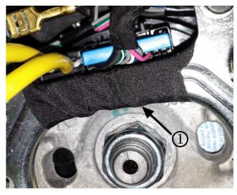
Note: After installing the protective material, verify the metal horn plate does not bind or stick as a result of the tape installation.
