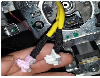
6. Wrap woven polyester electrical tape (PET) around each wire from the sleeve end toward the connector, to secure the sleeve from sliding back down.
