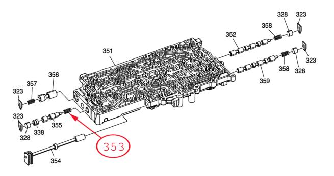
The root cause of this concern may be a broken torque converter clutch regulator valve spring (353) in the lower valve body, causing the torque converter clutch (TCC) slip speed to drop to zero.
