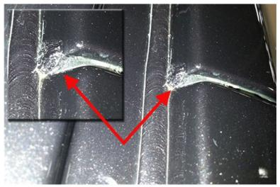
6 - With the roof rail removed on the affected side, inspect existing seam sealer in the area shown; door surround to quarter panel and roof panel (Area 2 as seen above) for skips or pin holes in the sealer.
