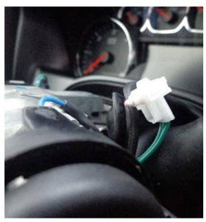
9. Install "short" key into ignition lock cylinder. If head of key bottoms out pull out slightly while applying front pressure to engage the tumblers.
