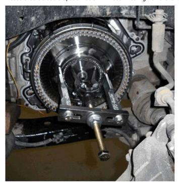
To install bearing use Special Tools DT-22928-B Seal Installer per SI, as damage may occur if the proper tools are not utilized.
