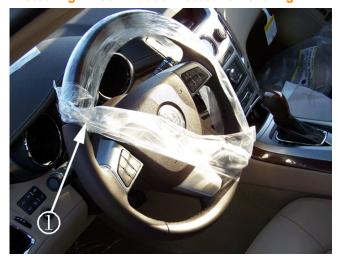
The removal process is quite easy. Sit in the driver's seat with your hands at the 11 o'clock and 2 o'clock position. Simply pull the plastic from behind, over the wheel toward you and then downward, taking care not to twist the plastic or allow it to bunch up.
