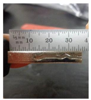
6. Then using a file/grinder, bevel the tip of the key in a similar fashion to the way it was from the factory. Also, grind / file the beginning of each groove so the tumblers will be funneled along the groove. Note: If this is not done correctly the key will only go into the lock cylinder part way.
