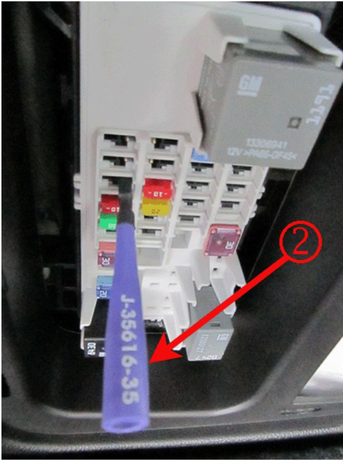
If poor terminal tension is found, first remove all the fuses and relays from the fuse block. Then, remove the white cover from the rear body fuse block (3) by releasing the three retainers on the sides and bottom.
