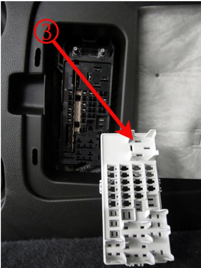
In many cases, the loose connection is on the main power buss bar, inside the rear body fuse block (4).
