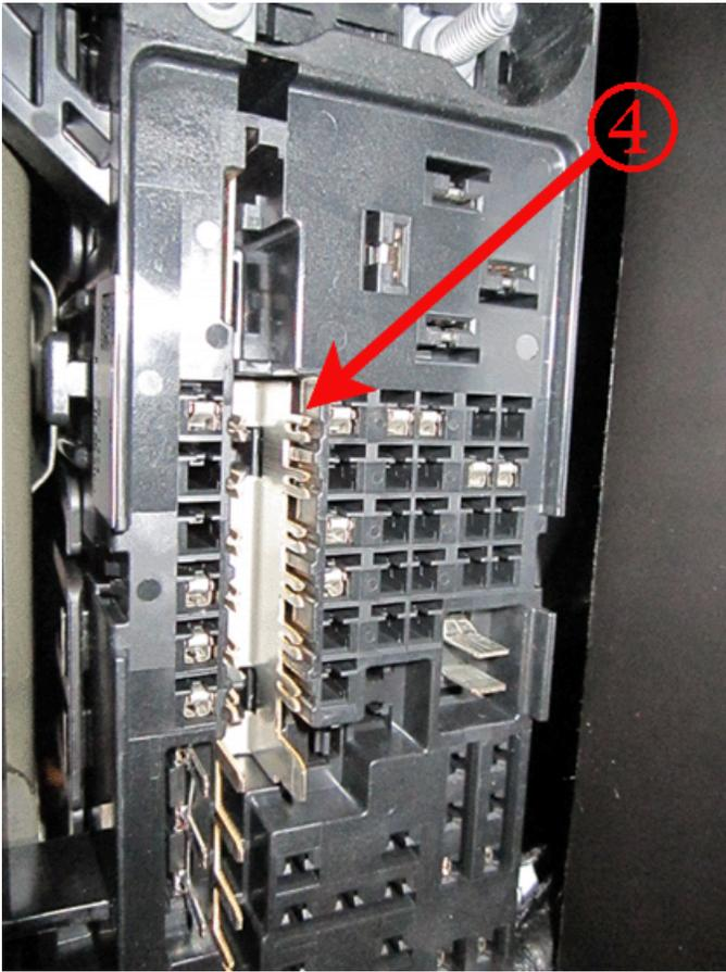
Using a pair of long nose pliers or similar tool, adjust the buss bar fuse terminal (5). Retest the terminal tension using the test probe and readjust if necessary until proper tension is achieved.
