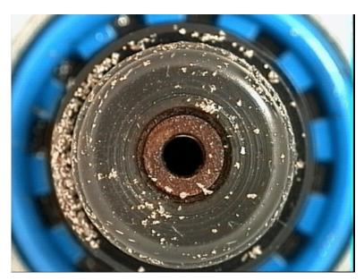
The pictures above are examples of Pressure Regulator 1 with the magnetic debris described
