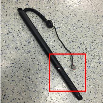
Note: The screw will hold the strut together for removal.
