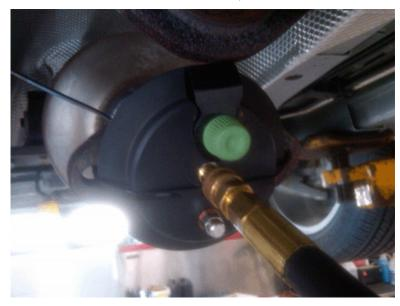
If a leak is found in these areas along with gasket replacement, filing the mating surface of the pipe is suggested.
