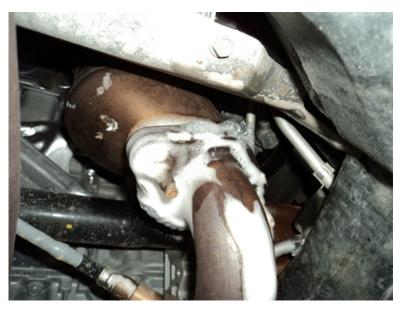
DO NOT APPLY FULL SHOP AIR as converter and engine damage can result.
