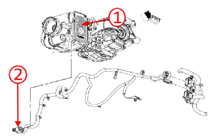
Inspect the K47 connector for corrosion/moisture. If corrosion/moisture has been found in the connector for the rear axle to suspension actuator wiring harness (2) and the rear differential clutch control module (RDCCM) (1), both components must be replaced.
