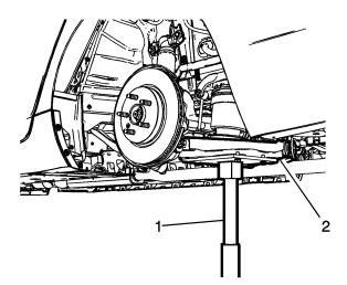
**13.** Support the rear cradle assembly with a support stand (1) or equivalent.
