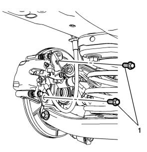
**Caution:** Support the brake caliper with heavy mechanic wire, or equivalent, whenever it is separated from its mount and the hydraulic flexible brake hose is still connected. Failure to support the caliper in this manner will cause the flexible brake hose to bear the weight of the caliper, which may cause damage to the brake hose and in turn may cause a brake fluid leak.
