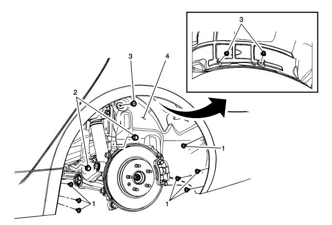
3. Remove the rear wheelhouse liner (4).
