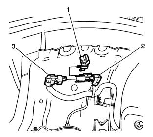
7. Disconnect the strut electrical connector (2) and separate the wiring harness from the body.
