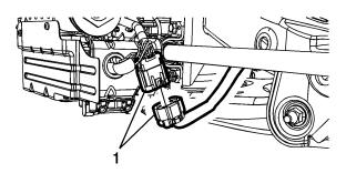
**12.** Disconnect the air ride pump electrical connector (1).
