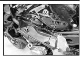
Side Cover Disassembly ● Remove the screws [A] and separate the covers [B].
