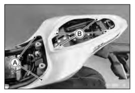
• Remove the seat cover [A] backward to clear the hooks [B].
