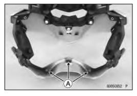
• Insert the tabs [A] and dampers [B] of the upper fairing into the slots [C] on the headlight unit.
