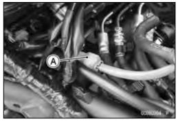
• Disconnect the fuel pump lead connector [A].
