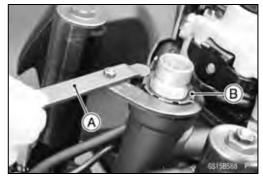
OYou may adjust the steering using the adjustable hook wrench [A].
