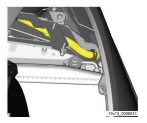
Open 2 cable clamps that holds coolant lines which are still connected then extract 2 pipes.
