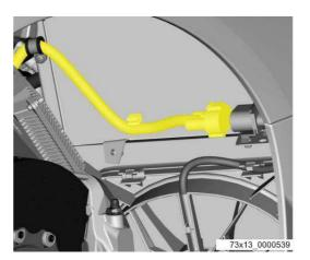
Open clamp that holds coolant line and then extract pipe.
