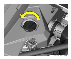
Prepare a suitable container to collect fluids, then remove coolant drain plug.
