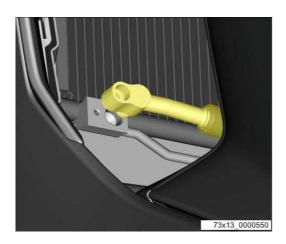
Now remove right radiator assembly that includes electric fan, cable clamp bracket, washers, spacers, buffers and condenser.
