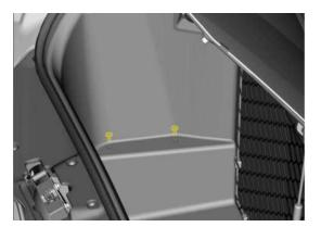
Lift trunk and disconnect plug from the 12V socket.
