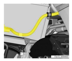
Open 2 cable clamps and extract 2 cooling pipes.
