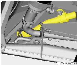
Remove screw that fixes hose clamp and then extract hose from cooler.
