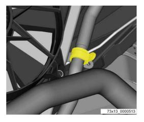
Remove 4 screws that hold left cooler group, free it from chassis then extract it from vehicle.
