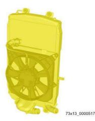
Now remove left radiator assembly that includes electric fan, cable clamp bracket, washers, spacers, buffers and condenser.
