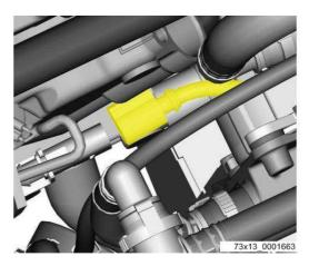
Disconnect connector of engine mounting and oil tank sensor.
