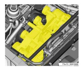
Pull two screws out from auxiliary support.
