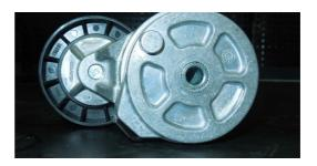
On old component is present a notch which is absent on the new one.
