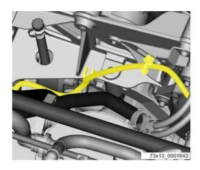
Remove screw, then free fuel cooler bracket of auxiliary mounting.
