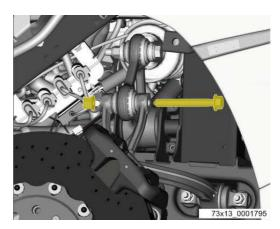
Unscrew nut and remove bolt that secure shock absorber.
