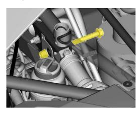
Remove shock absorber. Keep right and left wheel distinguished and during reassembly fit them with logo OHLINS pointing upward.
