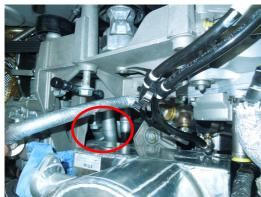
Free rear differential breather pipe and from clip and pull it out from hole onto aux. mounting.
