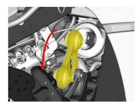
Unscrew nut and pull bolt out that fix shock absorber.
