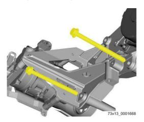
Remove spacer of aux. mounting.
