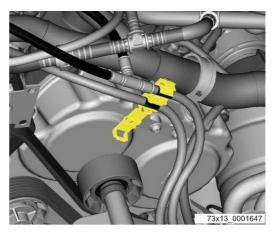
Remove screw which fix fuel line bracket so free auxiliary mounting bracket.
