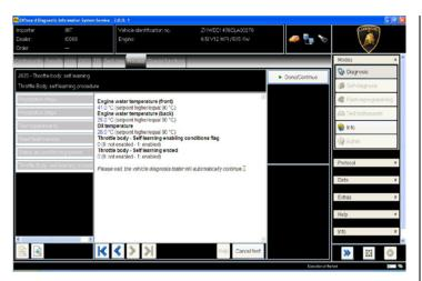
**78.** Once reached the activation conditions (water and oil temperatures major than 90°C) the "Throttle body – Self learning enabling con-ditions flag" changes from 0 to 1 indicating the start of the self-learning procedure.
