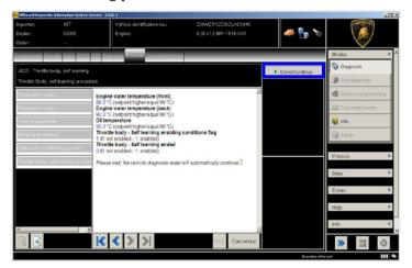
**79.** If the self-learning is completed successfully a screen as in the picture below is shown.
