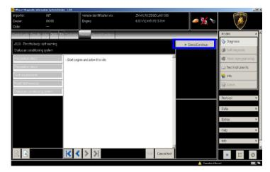
77. Self learning is an automatic procedure and it is activated when engine water and oil temperature exceed 90 °C.
