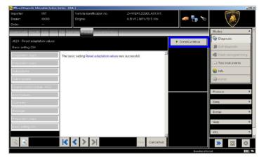
71. Go back to the Control Unit tab (block diagram or list view), to select the Engine ECU MOT\_01 and the Guided Function.
