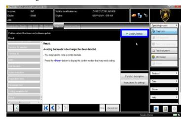
41. New coding has been calculated on control unit 17 - Instrument Cluster and it is necessary to write in the ECU.
