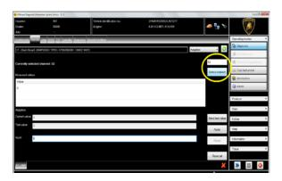
**89.** Insert the kilometers to the next service divided by 10 in the "Input" box (e.g if before the driveability package installation the remaining interval was 3400km, type "34", that is 3400/100).
