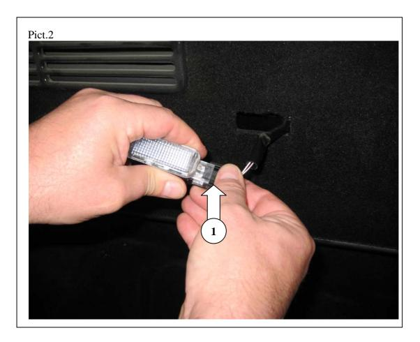
**1.4** Replace the old lamp housing (1-Pict.1) with the new lamp housing (p/n 3B0947415B).
