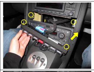
Align the seven switch console with the other items on the instrument panel.
