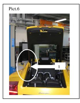
**2.6** Remove and replace the ETB ecu (p/n 400906018B) as explained at the points 1.3 and 1.5. Disconnect again the hydraulic engine bonnet (1-Pict.6) as explained at point 2.5. Reassemble the black cover (2-Pict.5) and the hydraulic engine bonnet (1-Pict.6) (workshop manual instruction 082705).
