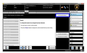
**28.** New coding has been calculated on the 17 – Instrument Cluster and must be written in the control unit.
