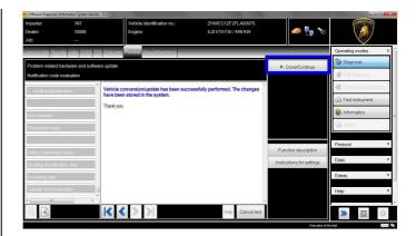
**40.** Once finished the update and quitted the software update (SVM) function, go back to the tab "Special functions" to select "Erase fault memory overall system": it is necessary to clear all the faults stored because of the recent software update.
