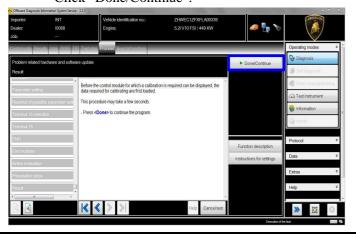
**35.** Continue with the calibration of the control unit 17 – Instrument Cluster
