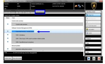
41. Execute the program "Erase fault memory – overall system" clicking on "Perform test..."
