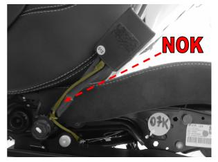
Remove the clamp on the buckle and release the electrical wiring.
