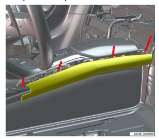
8. Remove the 2 clips that hold the carpet to the tunnel.
