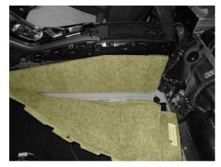
11. Lift the carpet from the car floor and slip off the seat wiring.
