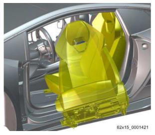
6. Remove the central tunnel soft cover leveraging the points indicated in the figure.
