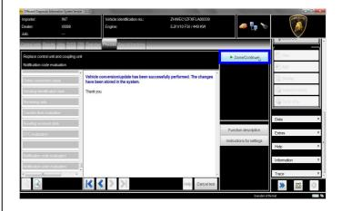
**36.** Once finished the update and quitted the software update (SVM) function, go back to the tab "Special functions" and select "Erase fault memory – overall system" to clear all the faults stored because of the recent software update.
