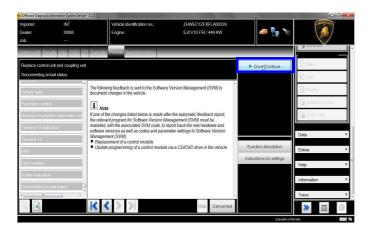
**34.** Wait until the data acquisition from all the control modules is completed.
