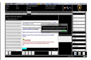
**21.** Once the update programming has been completed successfully a feedback as in the picture below is displayed.
