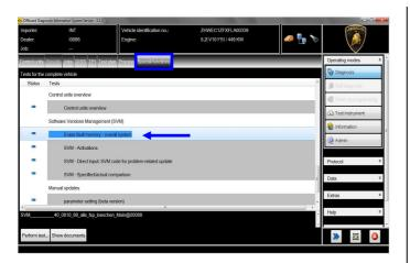
**37.** Execute the program "Erase fault memory – overall system" clicking on "Perform test..."
