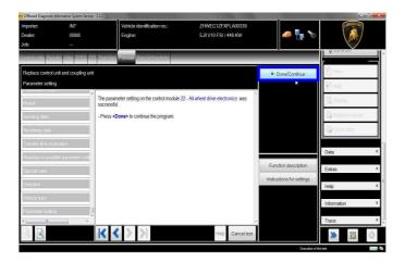
**29.** In the following an ignition OFF – ON cycle is necessary to restart both the ECU.
