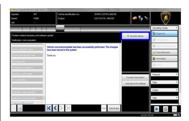
**39.** Once finished the update and quitted the software update (SVM) function, go back to the tab "Special functions" and select "Erase fault memory – overall system" to clear all the faults stored because of the recent software update.
