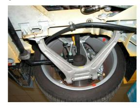
c) Underbody: general visual check on damages and loose parts
