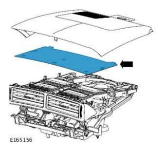
3. Install the instrument panel center vent (see TOPIx Workshop Manual, section 412-01). .
