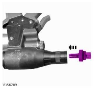
NOTE: The earth stud bond is totally selfsealing and watertight; there is no need to dress the hole with any primer before fitting.
