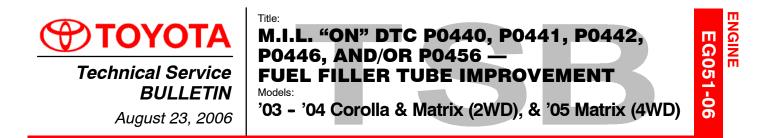
Introduction Some 2003 – 2004 Corolla and Matrix 2WD and 2005 model year Matrix 4WD vehicles may exhibit a M.I.L. "ON" condition with DTCs P0440, P0441, P0442, P0446, and/or P0456 stored. An improved fuel filler tube has been developed to correct this condition.
