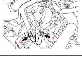
E. Disconnect the union to check valve hose from the intake manifold.
