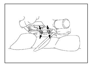
Without disconnecting the power steering fluid lines, remove the power steering pump.
