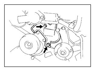
Repair Procedure (Continued) 10. Without disconnecting the A/C refrigerant lines, remove the A/C compressor from the mounting bracket.
