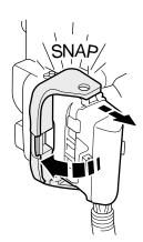
Open lever fully until it snaps before removing connector.
