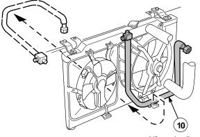
Lift suction line A from the bracket, and pull it out.
