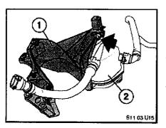
The new part has a cutout in the area of the coolant level sensor which eliminates the area of contact. Note area indicated by arrow.
