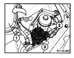
Remove the two bolts (2) securing the power steering reservoir (3). Position the reservoir away from bracket. Do not disconnect lines.
