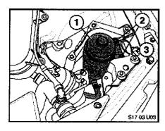
Remove the two bolts (2) securing oil filter housing (1) to bracket (3).
