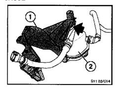
Insufficient clearance between underside of the coolant expansion tank (2) and the support bracket (1) as indicated by the arrow in illustration. Contact between the bracket and the coolant level sensor, located on the underside of the expansion tank, causes damage to the sensor which, in turn, leads to warning light illumination.
