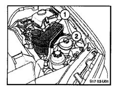
coolant expansion tank (1) as outlined in Repair Instruction 17 11 100. Tank is secured to bracket by two bolts (2)
