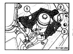
Remove the three bolts (2) holding the bracket (1) to the body. Carefully slide bracket around oil filter housing and remove. Install in reverse order.
