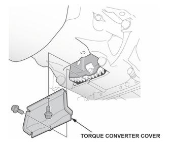
10. Rotate the crankshaft and remove all eight bolts.
