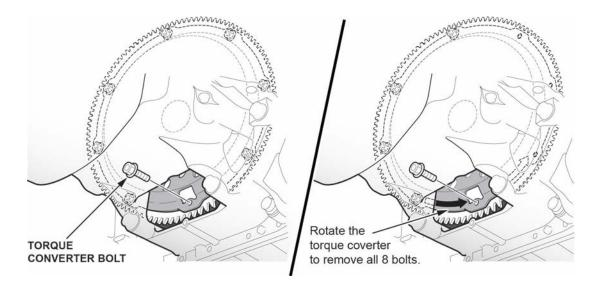
11. Rotate the torque converter clockwise one bolt hole. Then, install the bolts and torque them to **12 N·m (9 lb-ft)**.
