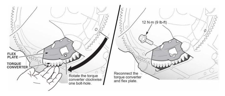
12. Mark the torque converter and the flex plate as shown. Then, write the bulletin number (16-016) on the flex plate with a permanent marker or paint marker.
