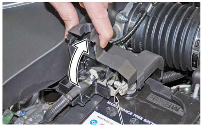
POSITIVE BATTERY TERMINAL
