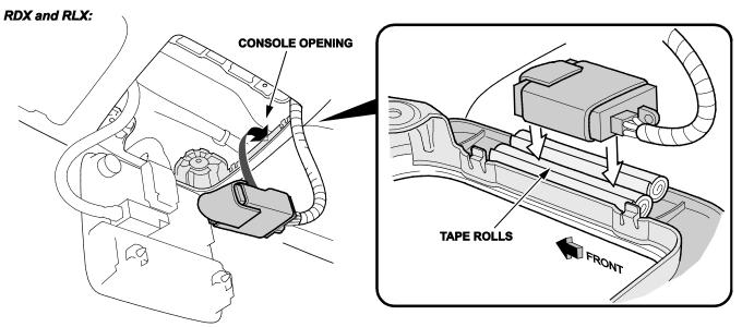
9. Secure the transceiver to the roof console with a white felt tape as shown.
