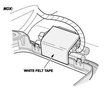
7. Stick the tape rolls to the console opening as shown.
