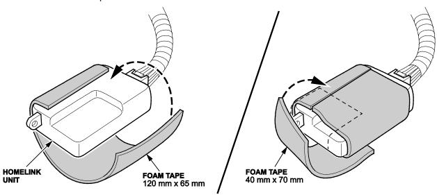
4. Remove the backing from two pieces of white felt tape and roll them up with the sticky side out. For MDX go to step 5 and for RDX/RLX go to step 7.
