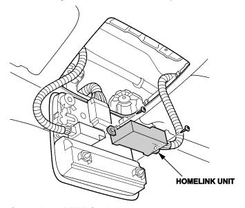
3. Cut a piece of EPT Sealer to 120mm x 65mm and wrap the entire HomeLink transceiver, then cut another piece 40mm x 70mm and wrap the end of the unit.
