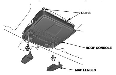
2. While holding the roof console assembly, remove the screws from the HomeLink transceiver.
