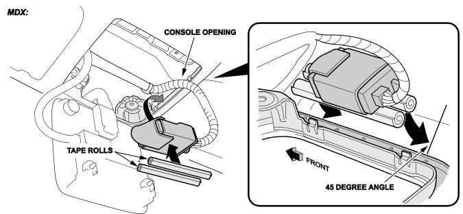
6. Secure the transceiver to the roof console with a white felt tape as shown.
