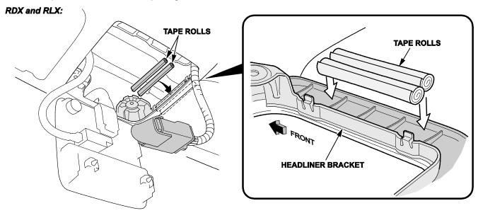
8. Stick the transceiver to the tape rolls with good pressure.
