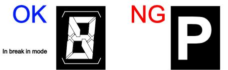
16. Start the engine. After about 10 seconds the break-in procedure will automatically begin and the Gear Position indicator will start to blink. This procedure takes about 4 minutes. During that time, engine fluctuation is normal. If you release the brake pedal or press down on the accelerator pedal, the procedure will stop and you will need to start over at step 3.
