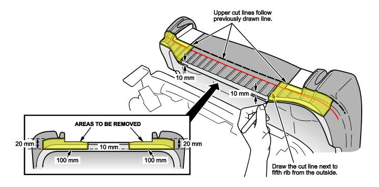
8. Carefully cut out the foam sections.
