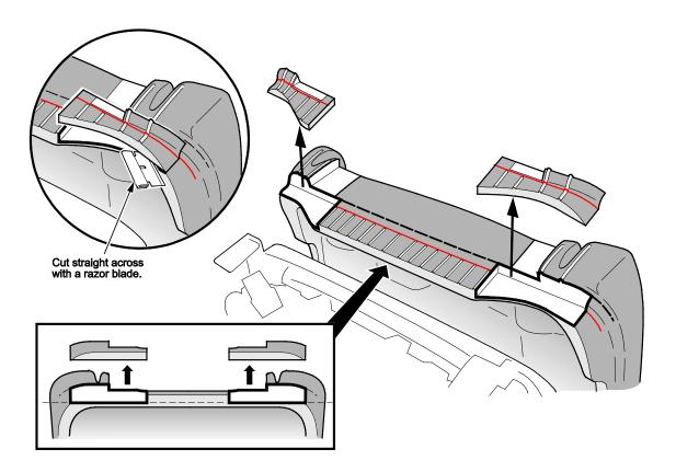
9. Carefully cut out the last foam section.
