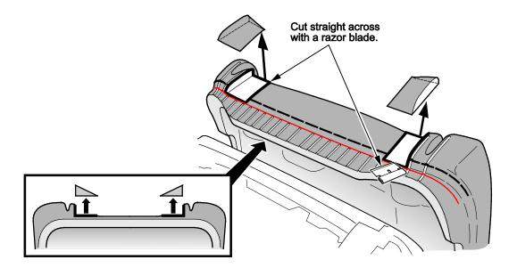
7. Use a felt tip pen to mark the front of the seat cushion as shown.
