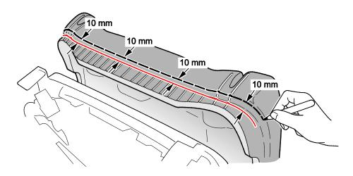
5. Use a ruler to measure and mark the seat cushion following the second rib lines as shown.
