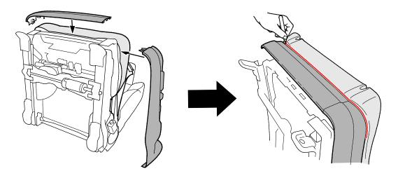
4. Remove the seat cushion and recliner covers, then use a ruler to mark a second cut line 10 mm above the reference line.
