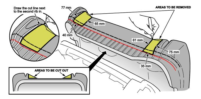
6. Carefully cut the foam sections out with a sharp razor blade.
