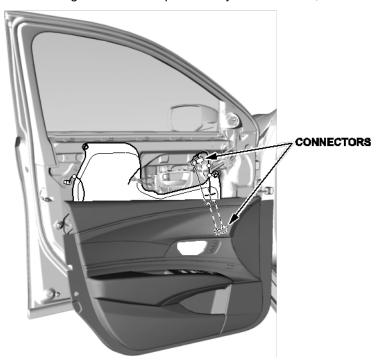
5. Disconnect the power door lock actuator connector and remove the harness clip.
