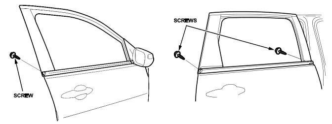
3. Starting at the rear, pull up on the door glass outer weatherstrip at each area where the inner molding catches the inside edge of the window slot.
