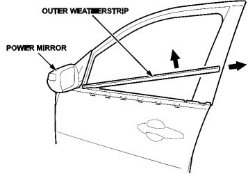
5. Using a utility knife, remove the entire lower seal from the molding.
