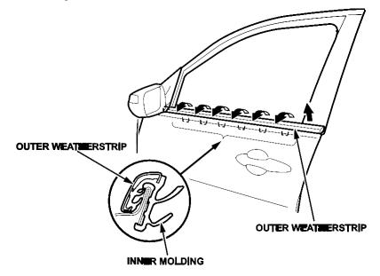
4. Lift the rear part of the door glass outer weatherstrip away from the door, then pull the front end of it out from under the power mirror.
