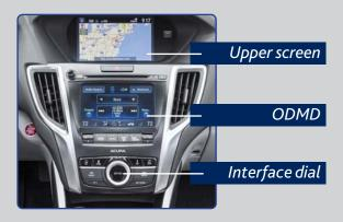
The upper screen displays audio, navigation, phone information, and more. Use the interface dial to control and operate this screen.
