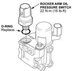
Install the new rocker arm oil pressure switch and the new O-ring. Torque the oil pressure switch to 22 N•m (16 lb-ft).
