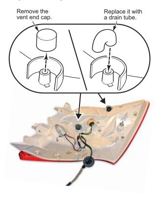
6. Install drain tubes where the two rubber vent caps were removed. After installing the drain tubes, make sure they face each other at about 45 degrees from vertical as shown.
