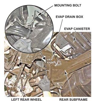
2. Pull down the drain box, then disconnect the fuel tank pressure (FTP) sensor vent hose from the drain box, and disconnect the EVAP vent hose from the EVAP canister.
