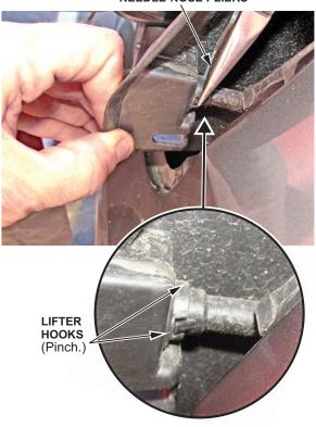
4. Install a new push lifter, push the adapter back into position, and reinstall the screw and the rubber push lifter cover.
