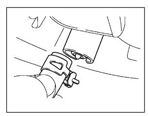
Push the drain hose up onto the evaporator drain tube. Ensure that the drain hose is up far enough for the retaining clamp to fully engage the tube.
