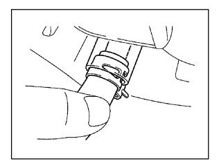
Repair Procedure (Continued) 4. Release the holding clip.
